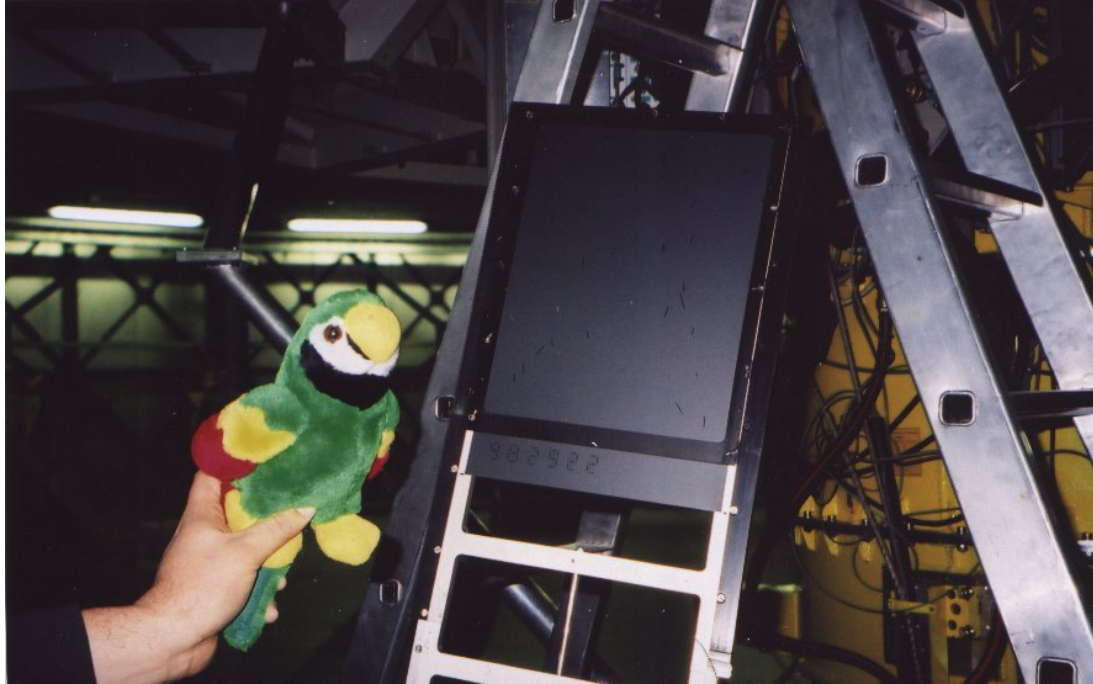
Figure 2.5: An MXU mask about to be inserted into the FORS2 instrument (partially visible behind the ladder). The parrot ‘supervising’ the procedure is the Nottingham astronomy mascot, Pepé ( http://www.nottingham.ac.uk/astrophysics/parrot/ ).
