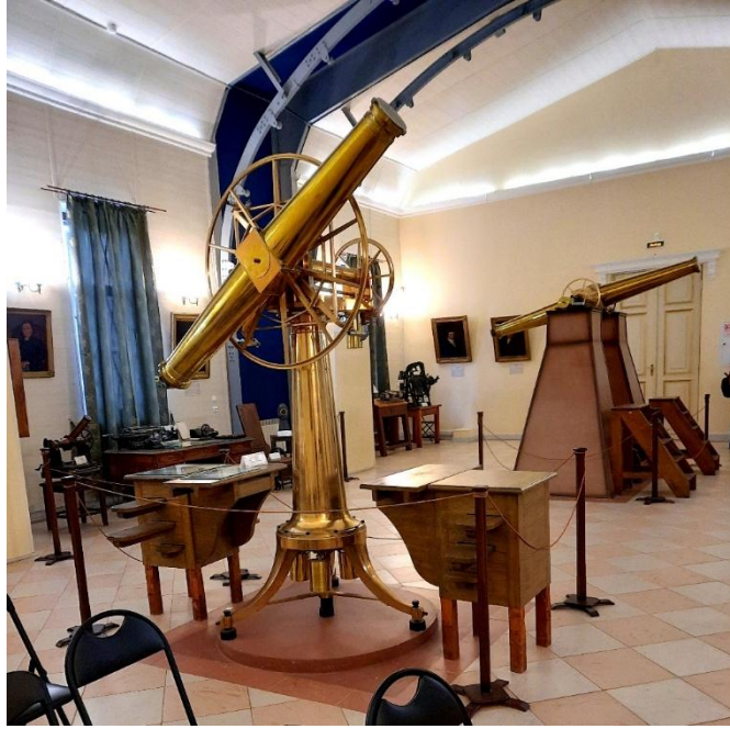
Figure 6. Classical Ertel-Struve vertical circle (in front) and transit instrument (behind) at the Meridian Hall of Pulkovo Observatory (converted to an astrometry museum). – Photo from 2024 by Vladimir N. Yershov.
